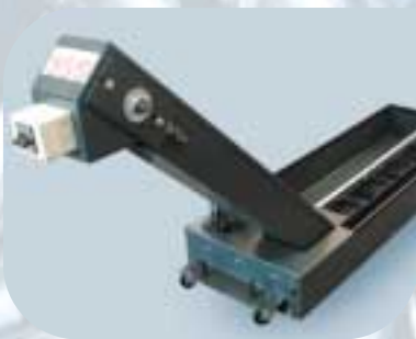
Flexible chip conveyor; can also be combined with interface for robot
