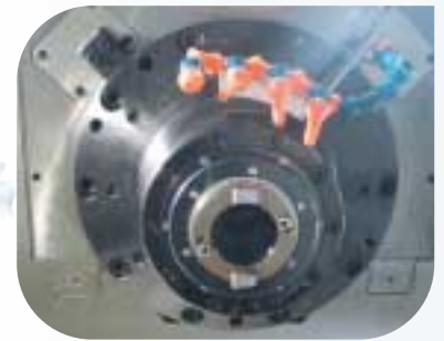
12,000 RPM spindle (ISO 40) with 4 adjustable coolant nozzles
