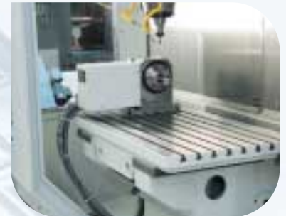
Dividing head in two sizes (VCP 600, VCP 800)
