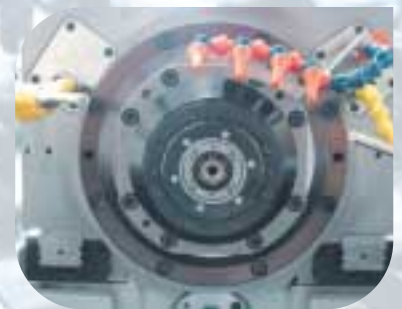
42,000 RPM spindle (HSK 40) with 4 adjustable coolant nozzles and 2 nozzles for minimum-quantity lubrication (optional)
