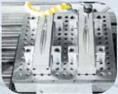
Multiple clamping increases the profitability of the production center
