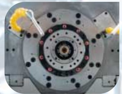
20,000 RPM spindle (HSK 63) with 9 coolant nozzles (distributed around the spindle center) and 2 nozzles for minimum-quantity lubrication (optional)
