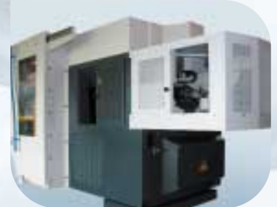
Expansion tool changer (ISO 40, HSK 63), total 58 positions (VCP 600, VCP 800, UCP 600)
