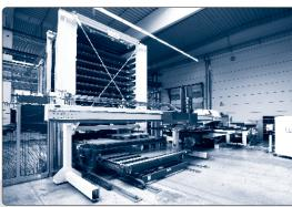
Connection of production machines with linear portal robotic loader
