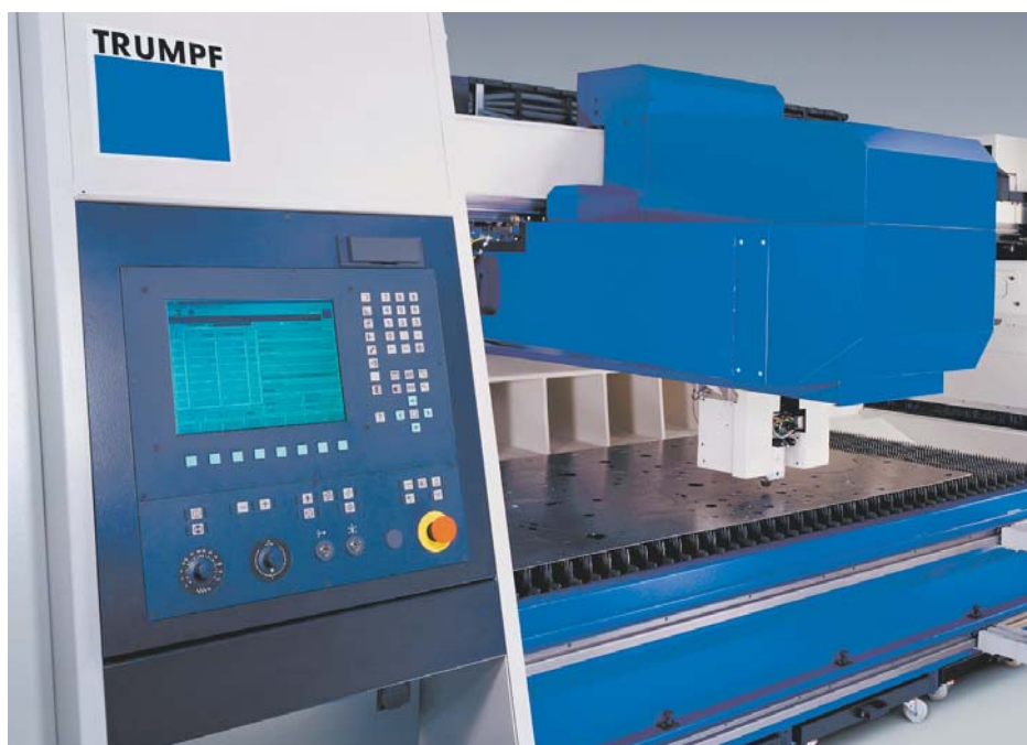
Operator panel in the machine frame.
