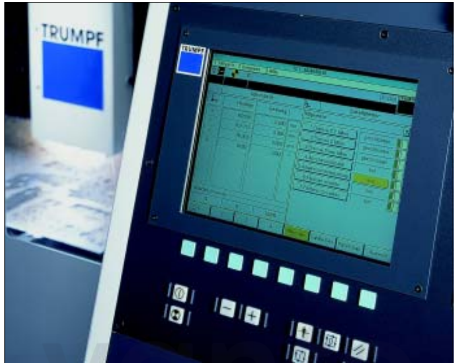
Operator panel in the machine frame
